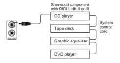
Connect this jack to the DIGI LINK jack of the external Sherwood component that uses the DIGI LINK II or III remote control system.
